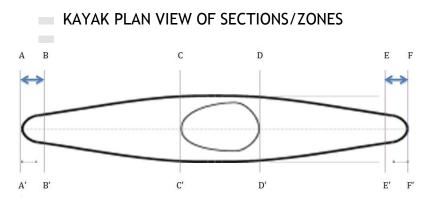
Section AA' to BB' - Front Impact Zone - measured to the point 100mm down the length of the kayak 100 mm minimum radius at any point on B-A-B'
