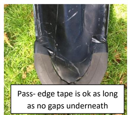
Any padding failing Step 2 must be replaced with a new padding of the appropriate type to suit the kayak design before it will pass. It is recommended that teams or individuals carry spare sets of padding for each design (Minor repairs can be completed during the event with tape or wrapping)
