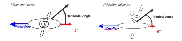
The 0° for the angle calculation is the long axis of the boat in a front or back surfing position.
