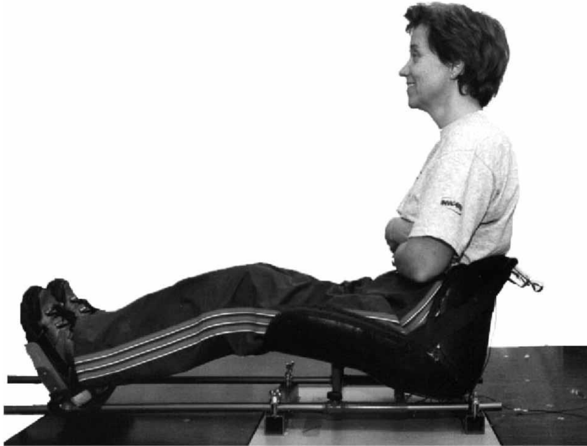
Fig. 1. The experimental set-up for balance testing. The subject is sitting in a special chair which is also used in the kayak. The chair is firmly attached to a force plate. The subject's feet are resting on a support connected to the chair via steel rods.
