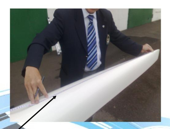
120 cms should be measure along the surface of a hull (the different shapes matters)
